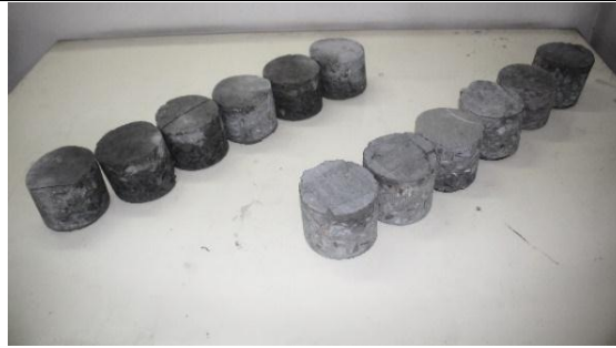
Figure 7: Core samples for pulse velocity test
