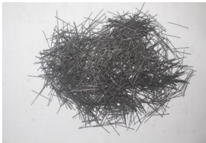
Figure 3: Steel fibres used in GPC-SF30
