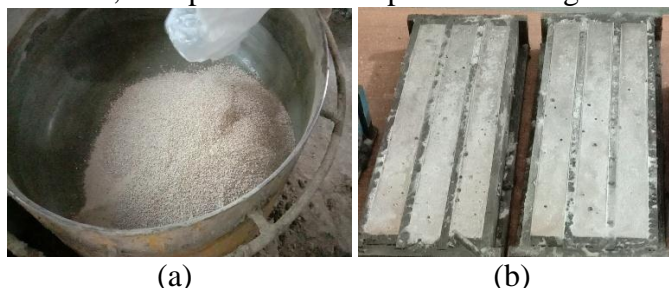
94 95 96 Figure 2. (a) Mortar Mixing, (b) Mortar bars before demolding
